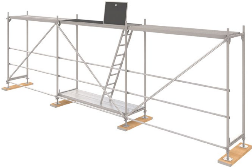
9.1.7 Steel decks and deck with ladders are mounted on the top profile of the main frame. The upper floor is accessed by using a ladder.
