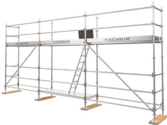
9.1.7 Steel decks and steel access deck with ladder are mounted and locked on horizontal braces. The ladder leads to the next floor. A safe working area is created by installing steel toe boards and horizontal braces.
